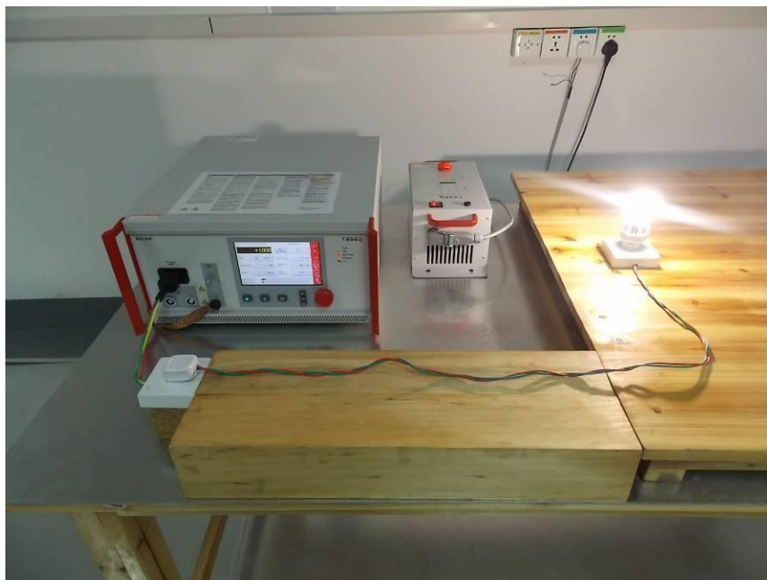
Photograph 6: Set-up for Fast Transient Burst & Voltage dips and interruptions to AC Power Port
